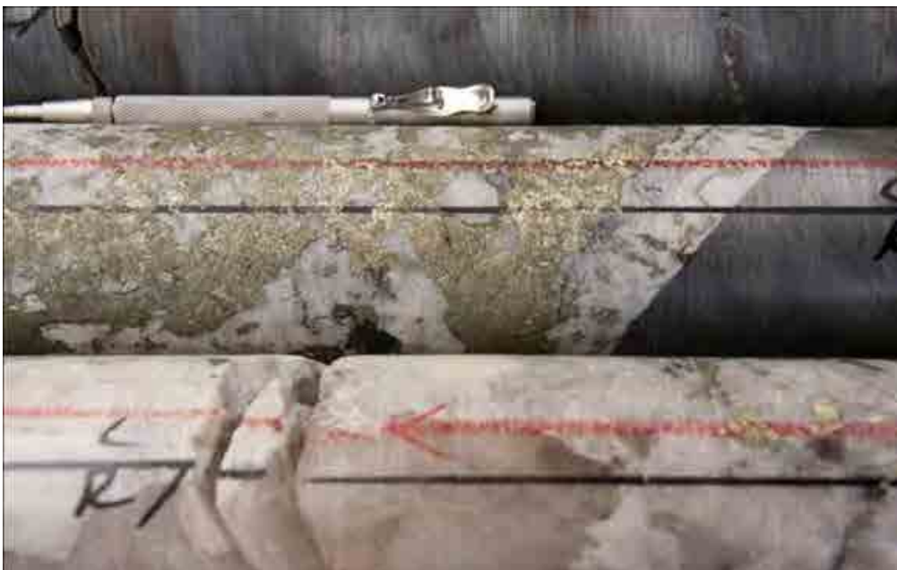
Figure 7-7 Vein hosted copper mineralisation in a fresh sulphide zone at Kansanshi
