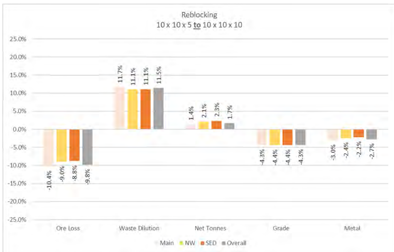
Figure 15-1 Impact of model reblocking to 10m x 10m x 10m resolution
