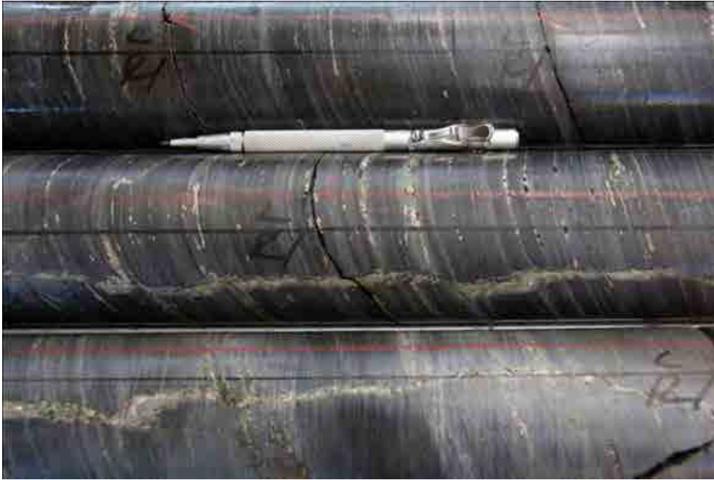
Figure 7-6 Stratabound and stringer veinlet mineralisation within a carbonaceous phyllite
